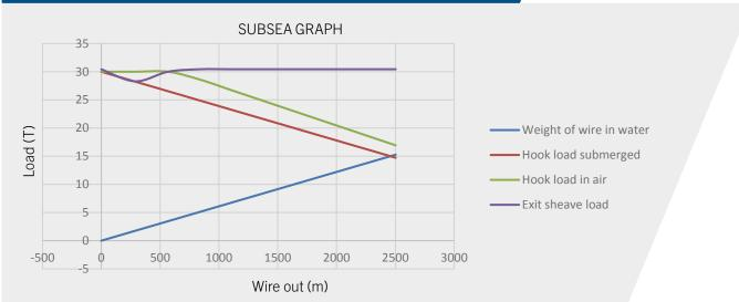
"Hook load submerged" is the maximum allowed force that can be applied in the hook at this depth.
